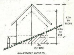
wall height of 4.5 metres and a gable height of 6.0 metres measured from natural ground level and finished ground level.
